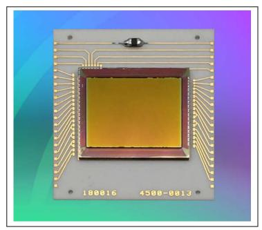
combined with the high quantum efficiency of the lattice matched InGaAs detector arrays enables impressive imaging in the SWIR and visible bands. Princeton Infrared Technologies, Inc. offers this low power array by itself on a ceramic submount or with a custom packaging. It is also incorporated in a set of camera electronics for a complete solution in our 1280SciCam.
