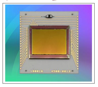
combined with the high quantum efficiency of the lattice matched InGaAs detector arrays enables impressive imaging in the SWIR and visible bands. Princeton Infrared Technologies, Inc. offers this low power array by itself on a ceramic submount or with a custom packaging. It is also incorporated in a set of camera electronics for a complete solution in our 1280SciCam.
